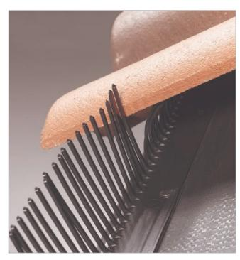
The Eaves Filler Comb is a simple and effective way of preventing birds and vermin from entering the batten cavity below profiled concrete interlocking tiles whilst allowing airflow into the batten cavity.
